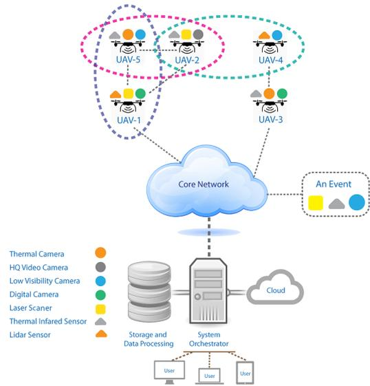
Fig. 1. UAV network architecture and equipment-based UAV set selection.
