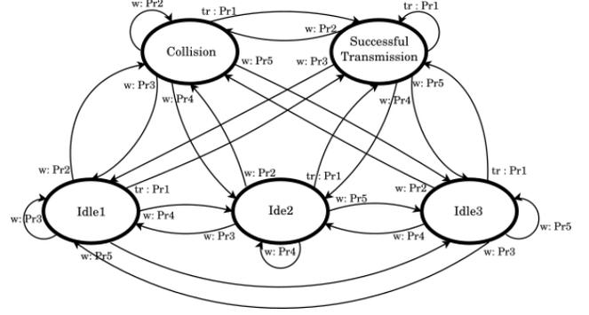
Fig. 1: MDP of collision handling at the wake-up plane
