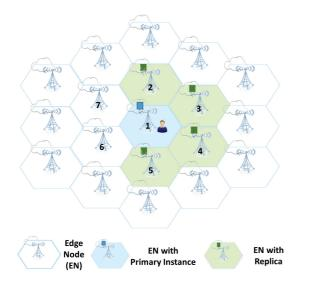
Fig. 1. Example deployment of proactive migration based on replication.
