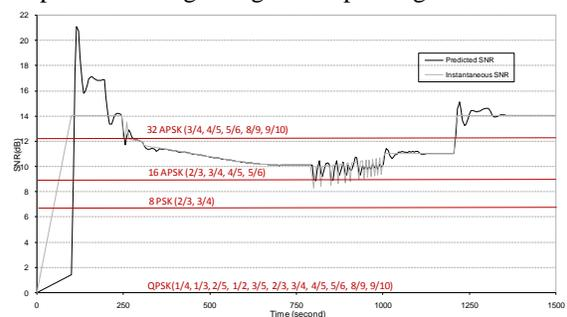
**Fig. 4** The instantaneous SNR vs the predicted SNR. Fig. 4 shows the instantaneous SNR experienced by a satellite terminal versus the predicted SNR. In the first stage of the simulation, we observe that the estimation error is relatively important. This is principally due to the random initialization used in Least Mean Square (LMS). After 105 seconds, we clearly see that the estimation becomes more precise which demonstrates the effectiveness of our proposed
