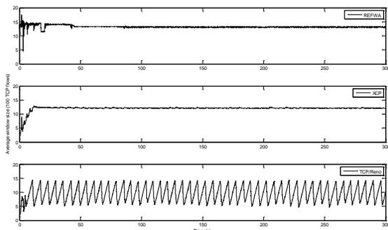
Fig. 2 The average window size for REFWA, TCP and XCP.
