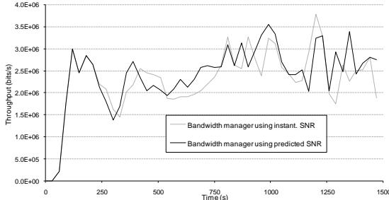
**Fig. 5** Throughput using instantaneous vs predicted SNR. Fig. 5 indicates the performance of the proposed mechanism in terms of throughput. The figures clearly shows that the bandwidth manager using predicted SNR values, which allow selecting the appropriate modulation and code rate, outperforms the conventional approach. As a consequence, the experienced throughput is increased by approximately 4.6%.
