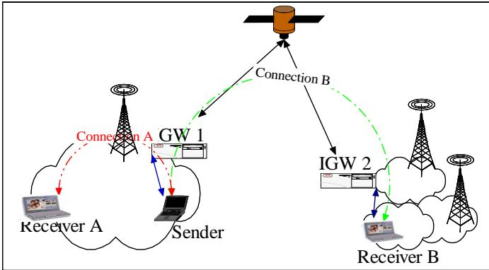
**Fig. 1** RTT-based Connection Setup + Connection Decoupling
