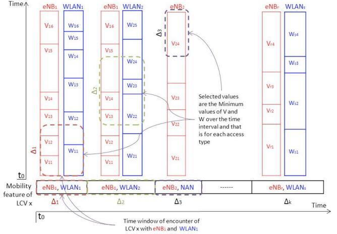
Fig. 4. Envisioned matrix for comparing QoE to be perceived at different access points of different access types a vehicle would encounter during a time window of interest.
