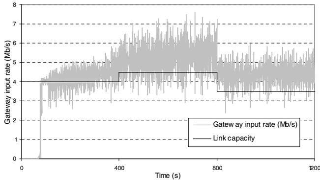
Fig. 6. DVB-S2/DVB-RCS Gateway input rate in case of only uplink CAC (MPEG2-TS level).
