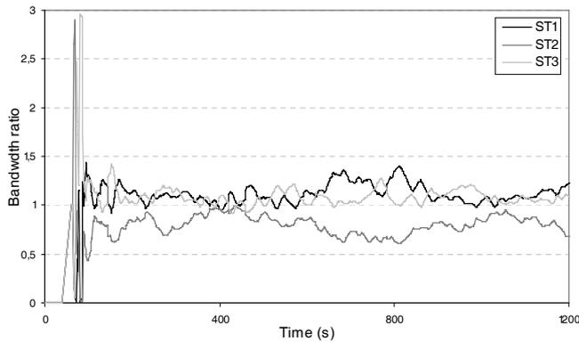
Fig. 10. Average received bandwidth ratio in case of W-FCAC (IP level).
