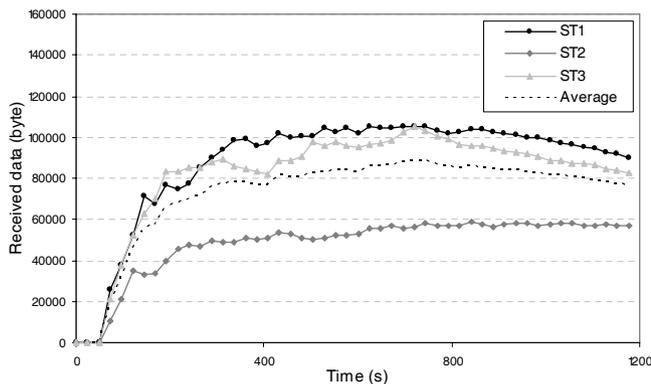
Fig. 11. FTP clients received bandwidth in case of only uplink CAC (Application level).
