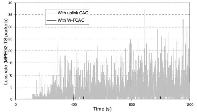
Fig. 8. Loss rate variation in case of only uplink CAC and W-FCAC (MPEG2-TS Level).
