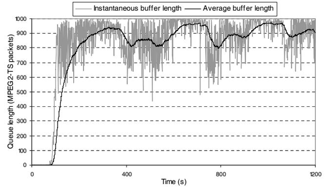
Fig. 4. Variations of the downlink queue length in case of only uplink CAC (MPEG2-TS level).
