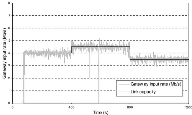
Fig. 7. DVB-S2/DVB-RCS Gateway input rate in case of W-FCAC (MPEG2-TS level).
