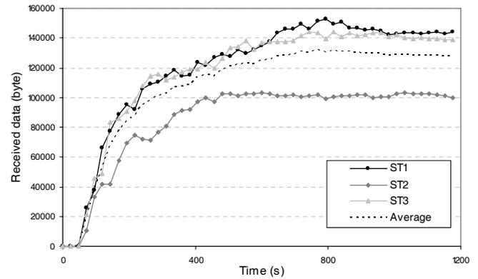
Fig. 12. FTP clients received bandwidth in case of W-FCAC (Application level).
