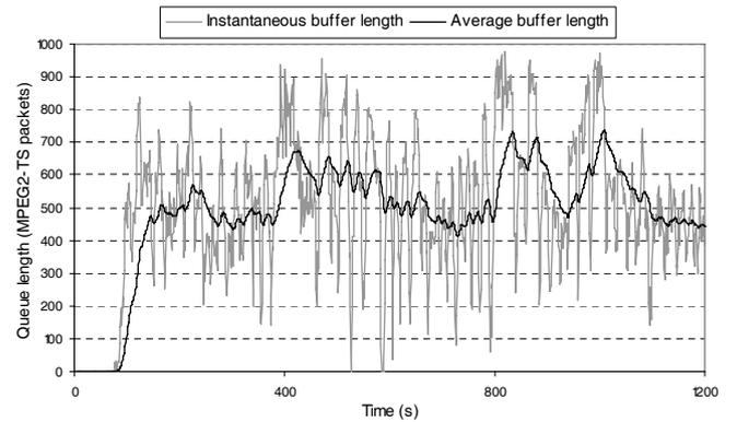
Fig. 5. Variations of the downlink queue length in case of W-FCAC (MPEG2-TS level).
