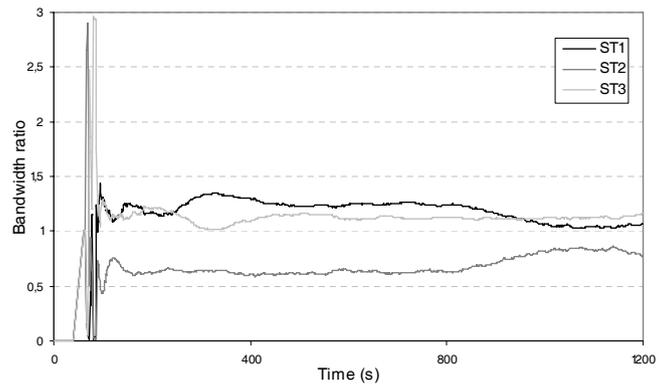
Fig. 9. Average received bandwidth ratio in case of only uplink CAC (IP level).
