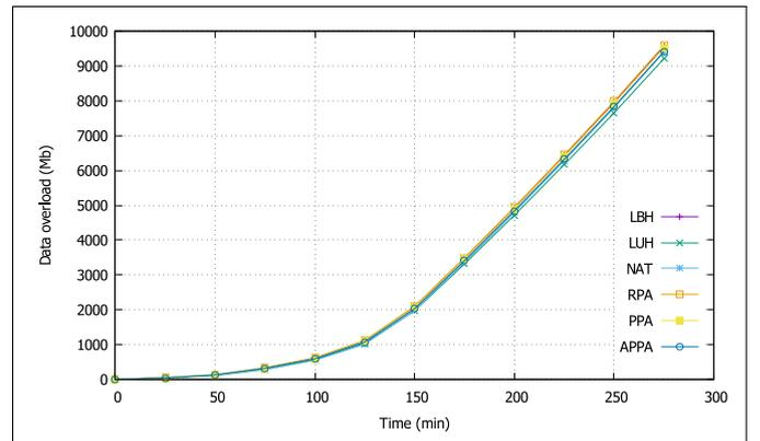
Fig. 3: Data overload of different VNF placement strategies.
