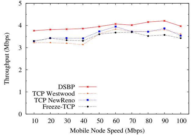
(a) Case I: Handoff from a low bandwidth cell (6 Mbps) to a high bandwidth cell (11 Mbps)
