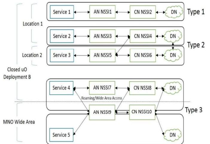
Fig 6. Deployment B: One closed network for multiple locations.
