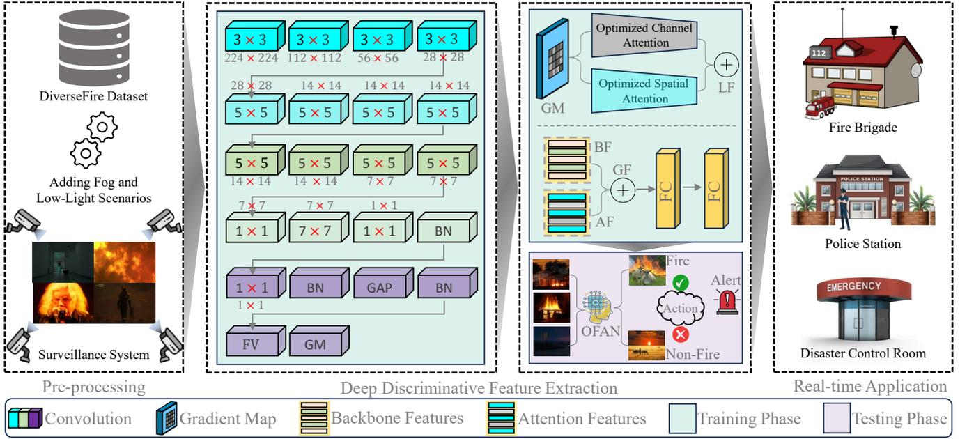
Fig. 2. The proposed *OFAN* framework: Enhancing fire detection with deep discriminative feature extraction, optimized attention mechanisms, and synthesized *DiverseFire* benchmark.
