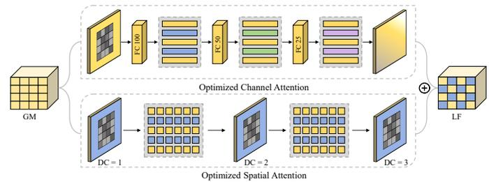
Fig. 3. Block diagram of a modified attention block, where fully connected (FC) and dilated convolution (DC) with variable dilation rate are employed to extract more prominent features from the given gradient map (GM). Furthermore, parallel attention feature maps are integrated as local fusion (LF).
