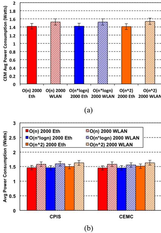
Fig. 9. Power consumption (a) of the CEM, and (b) of the device hosting the CoAP server for different computation tasks.
