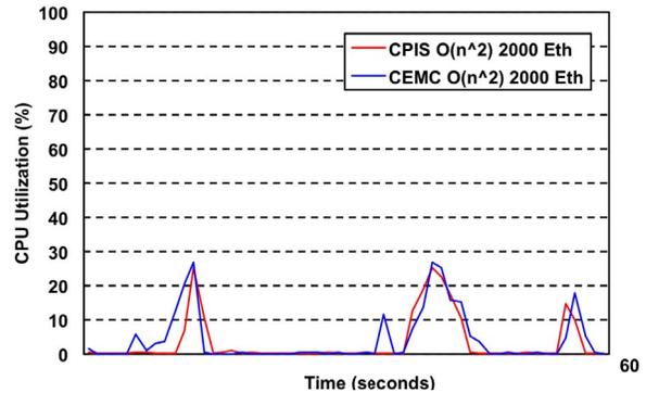
Fig. 8. Comparison of CPU utilization of the device hosting the CoAP server for a computation use case accounting for both CPIS and CEMC modes.
