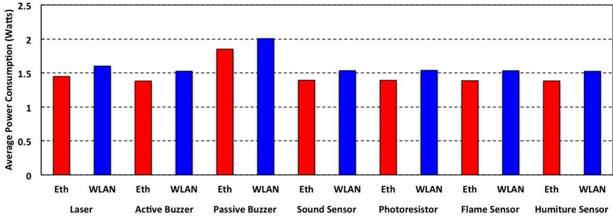
Fig. 11. Average power consumption for sensing/actuation scenarios, in both Ethernet and WLAN configurations.
