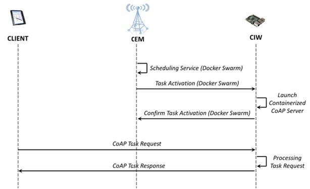
Fig. 3. Workflow of CEMC for clustered IoT environment.
