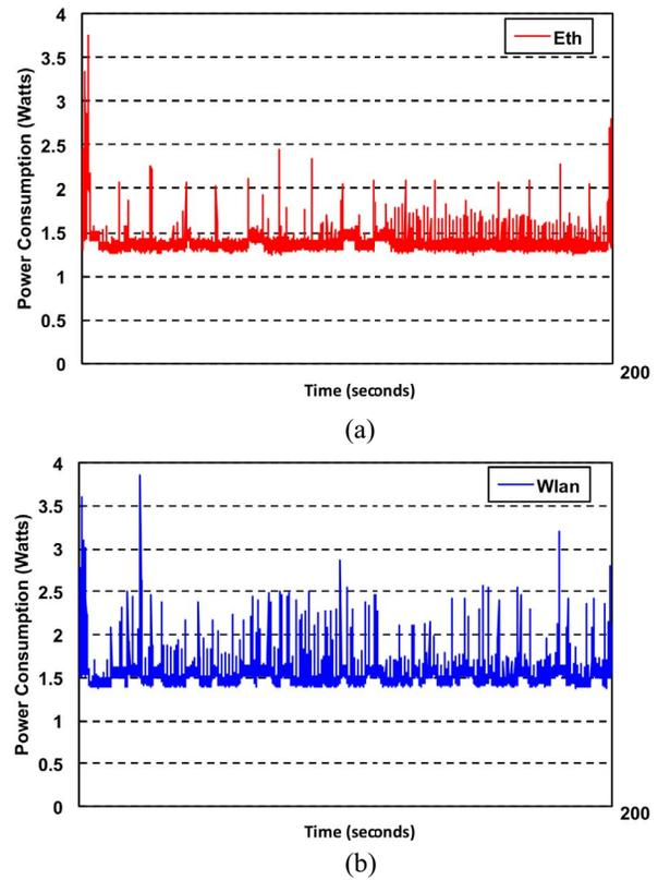
Fig. 12. Power consumption of the device running the Docker containerized CoAP server for active buzzer in (a) Ethernet configuration and in (b) WLAN configuration.
