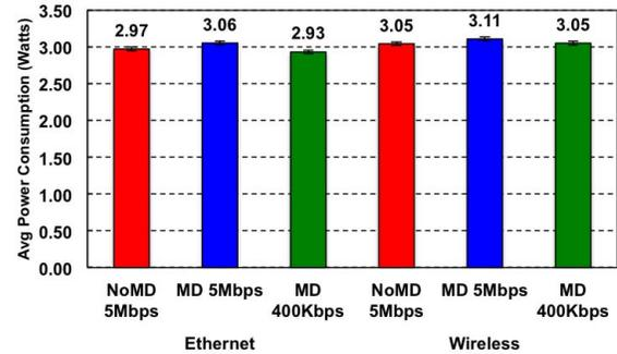
Fig. 15. Average power consumption of Docker containerized video services with/out motion detection (MD) filter.
