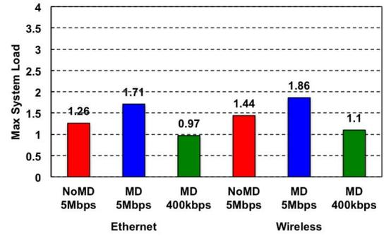
Fig. 14. Max system load of Docker containerized video services with/out motion detection (MD) filter.
