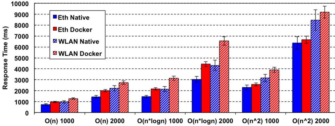
Fig. 5. Response times of computation tasks for different input sizes, comparing the native case to the Docker containerized services, in both Ethernet and WLAN configurations.
