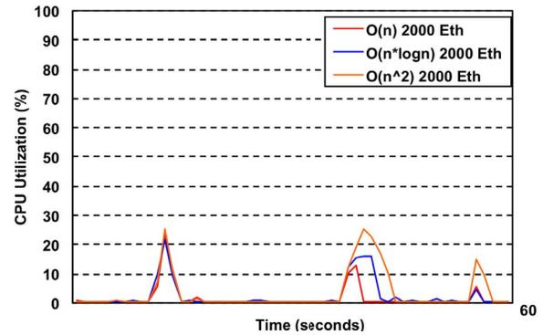
Fig. 7. Comparison of CPU utilization of the device hosting the CoAP server for different computation tasks in CPIS mode.
