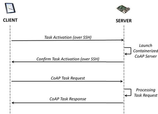
Fig. 1. Workflow of the CPIS approach for clustered IoT environment.
