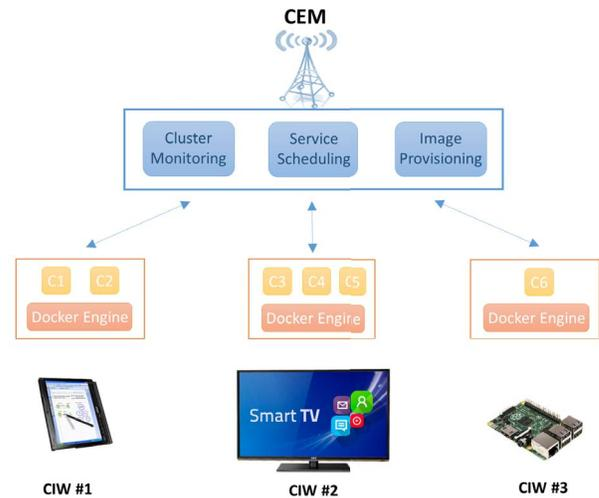
Fig. 2. Container-based architecture for clustered IoT environment.
