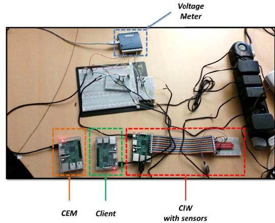
Fig. 4. Testbed environment for CEMC approach in wireless configuration.
