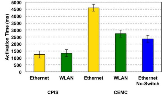
Fig. 10. Activation times of Docker-based containers for different configurations.
