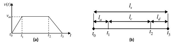
**Fig. 1: (a) Simplified velocity function and (b) Association between time and length of a road segment portion.**
