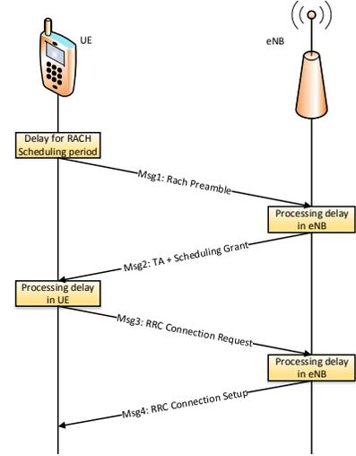
Fig. 2. Random Access CHannel (RACH) procedure
