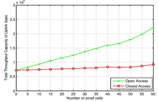
Fig. 3. Total throughput capacity of uplink.
