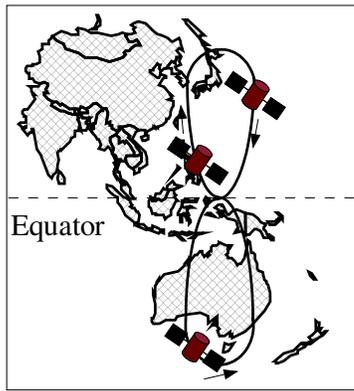
Fig. 1. An example of a Quasi-GSO satellite system made of three satellites
