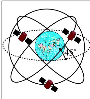
Fig. 2. Circular orbits of Quasi-Geostationary satellites
