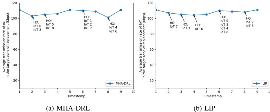
Fig. 4: Evaluation of the UAV-BS replacement process for the proposed MHA-DRL against LIP (optimal solution).
