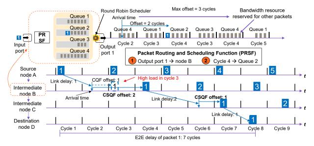
Fig. 1: CSQF-based cycle scheduling of a DN flow.
