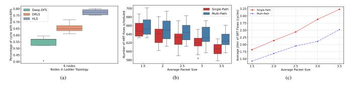
Fig. 5: (a) Percentage of cycles with traffic load over 60%; (b) Number of HRT flows scheduled under single and multi-path scheduling; (c) Average jitter of SRT flows under single and multi-path scheduling.
