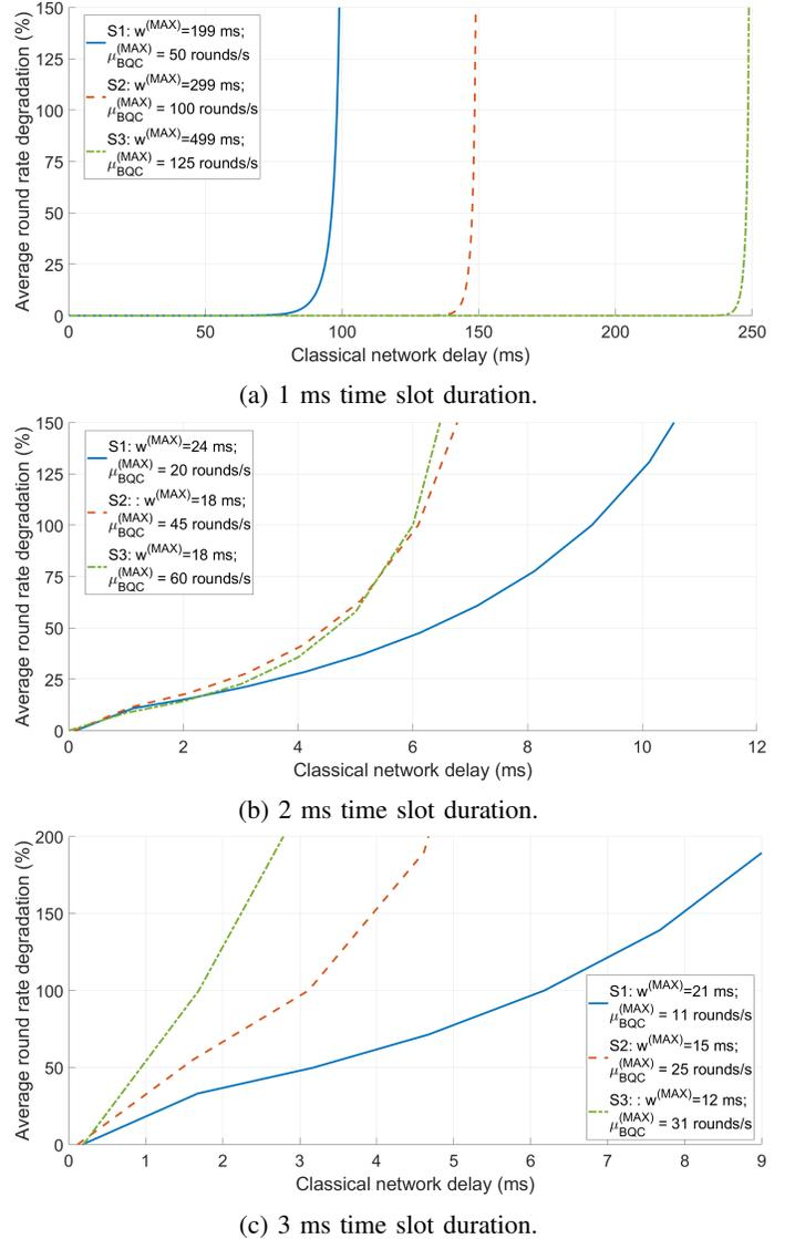
Fig. 5: Two-qubits blind quantum computing service performance degradation versus the classical network delay to assist the quantum teleportation process.
