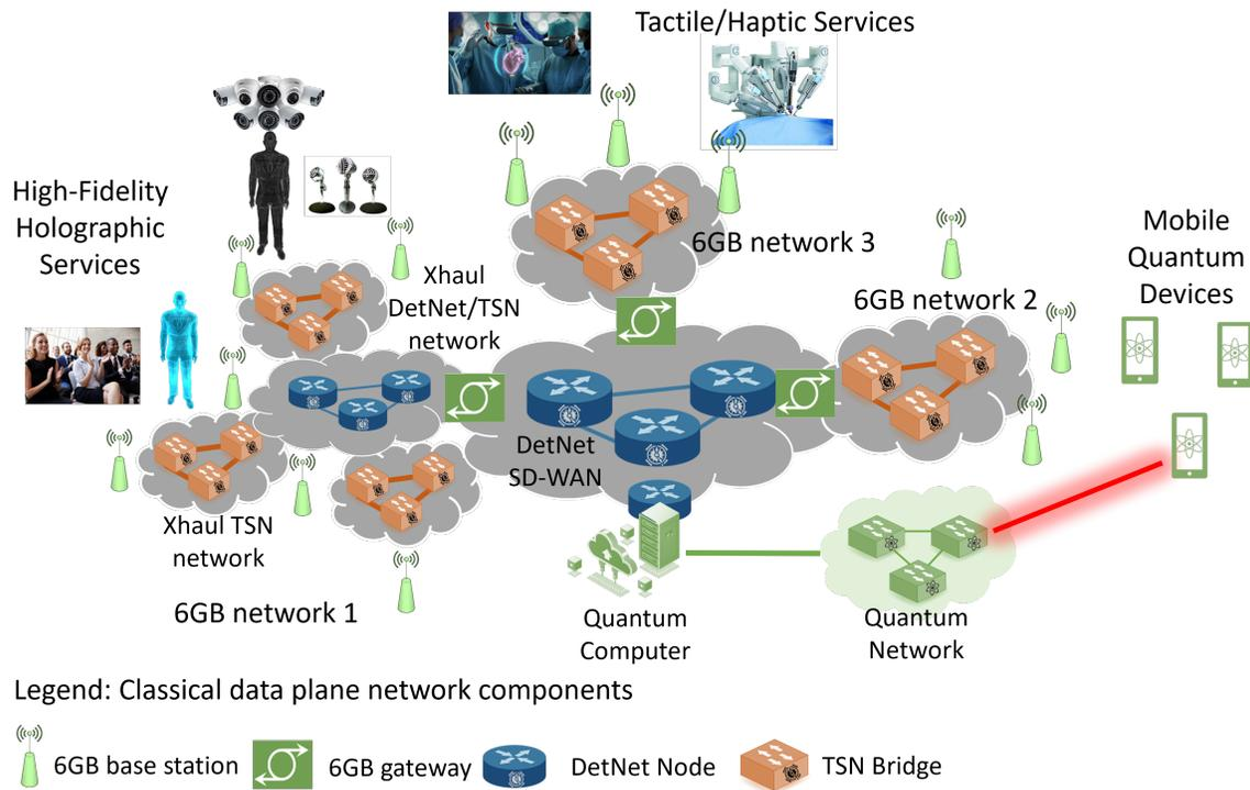
Fig. 2: Seamless integration of 6GB with TSN and Detnet data planes to provide long-range and truly end-to-end ultra-reliable low-latency connectivity for high-fidelity holograms, tactile/haptic and quantum services.
