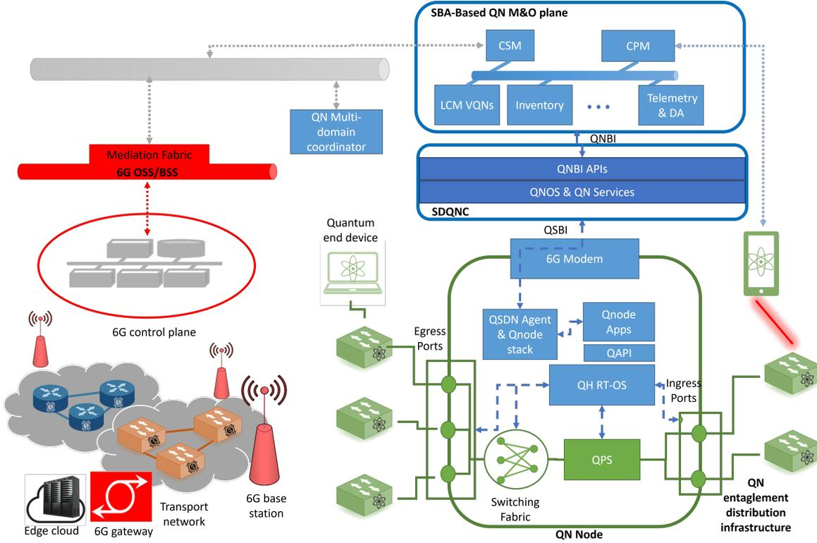
Fig. 4: Software-Defined programmable quantum network leveraging 6GB connectivity, exposure of management, synchronization and positioning services.
