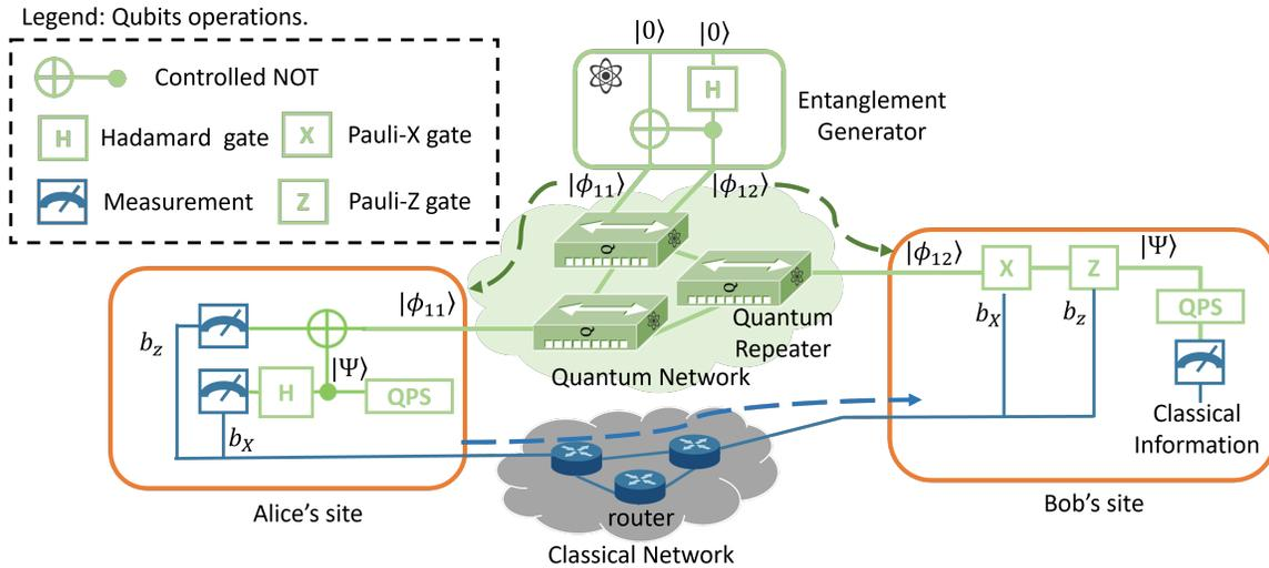
Fig. 1: Quantum network model and qubit teleportation process.
