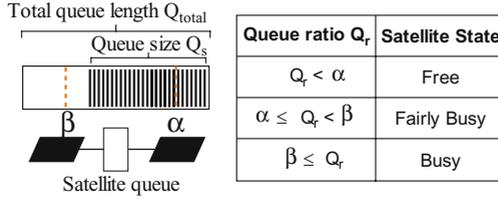
Fig. 1. The three network states of satellites
