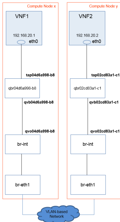
Fig. 5. Standard OpenStack network communication diagram
