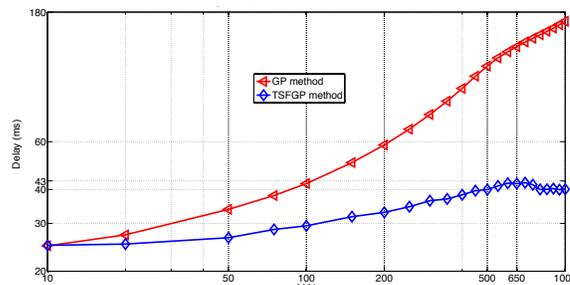
Fig. 5: The average access delay in case of both GP and TSFGP.
