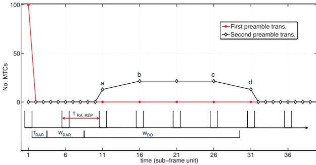
**Fig. 1:** Number of MTC devices at each RA slot for the first and second preamble transmissions for the considered parameters.
