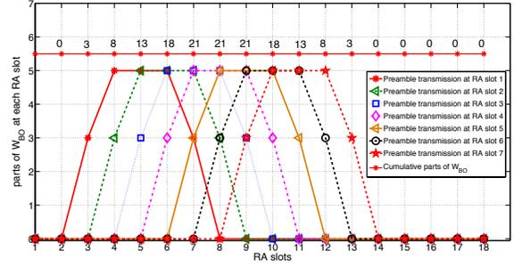
**Fig. 2:** The cumulative parts of  $W_{BO}$  for each RA slot for MTC devices transmitting their preambles for the second time, where  $W_{BO} = 21$  and  $T_{RA\_REP} = 5$ .
