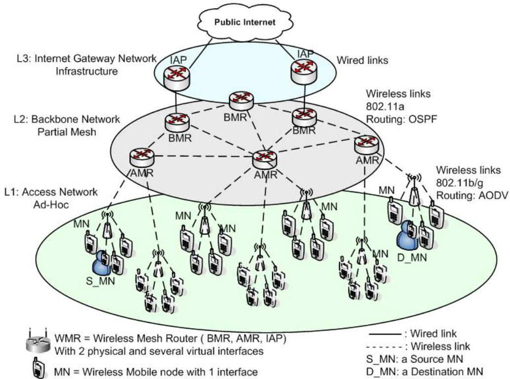
**Figure 1: Wireless mesh network baseline architecture.**
