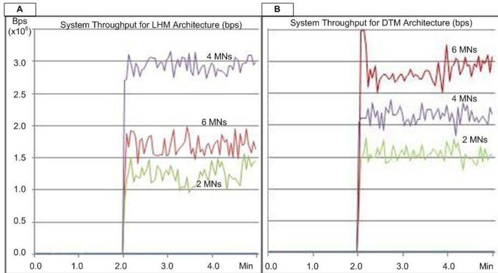
**Figure 5: Overall system throughput for LHM (A) and DTM (B) Architectures.**
