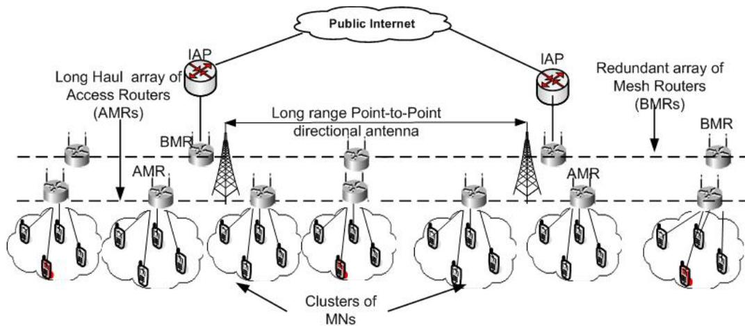
**Figure 4: Long haul mesh architecture.**
